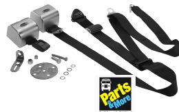
Q8-6326-A2 TWO RETRACTORS FOR LAP/SHOULDER BELT, 1 EXTENSION, 2 PIN CONNECTORS.
