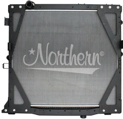
238799 RADIATOR 35 1/8" X 40 1/8" X 2 1/16" (PTR WITH FRAME)
