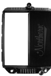
238505 RADIATOR FITS BLUEBIRD & INT'L 31" X 12 2/4" X 1 9/16"
