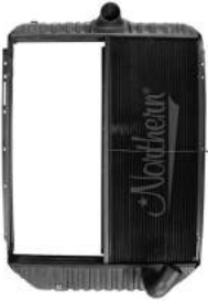
238555 RADIATOR FITS BLUEBIRD & INT'L 31" X 12 3/4" X 2 1/16"
