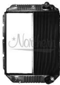
238565 RADIATOR FITS BLUEBIRD & INT'L 31" X 12 3/4" X 2 1/16"
